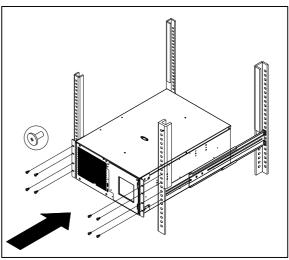
Take the rack mount rail inscribed with an "L" (Left) and attach it to the rear bracket of the Rack-mount Rail using three (3) of the six (6) Rack-mount Rail Screws. Do not fully tighten the rack mount rail screws, as the rack mount rails will need to be adjusted to fit your rack. Once complete, perform the same steps for assembling the Rack-mount Rail inscribed with an "R" (Right).
